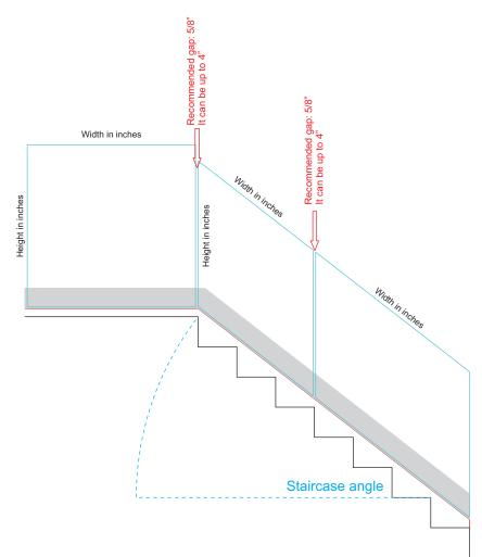
NOTE: Standard glass height to meet Code on the stairs: 34" to 38" from the nose of the thread. That's usually the height of the panel itself.
