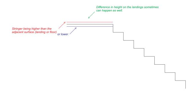
In the example below, we have a stringer that is 2" higher than the staircase (measuring at the nose of the thread) and the same 2" higher than the adjacent base at the landing:
